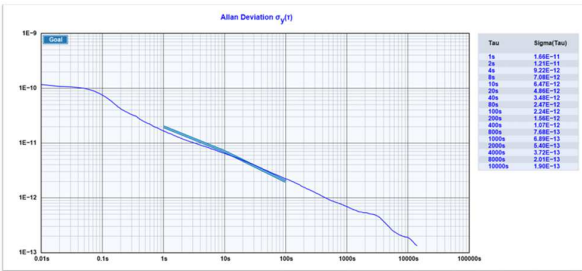
Figure 10: ADEV of prototype 8300C
